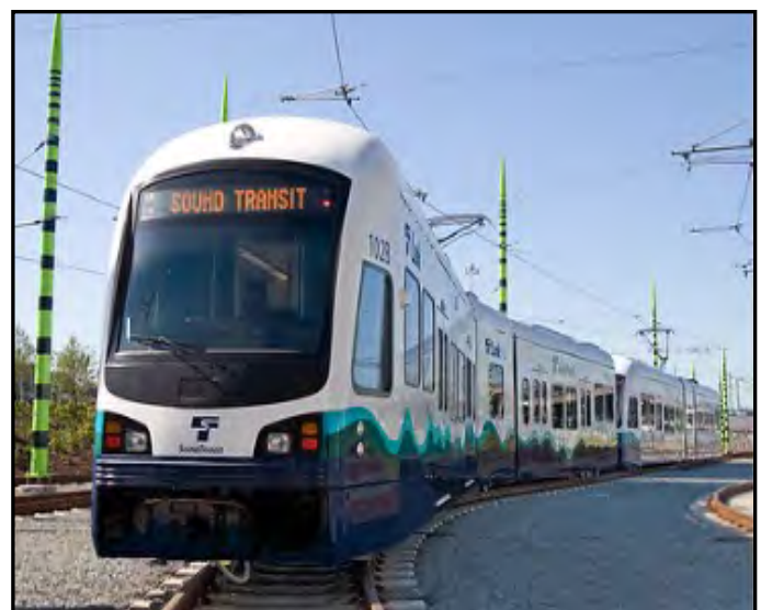
Light Rail Train run by the Overhead Catenary System (OCS) powered from the Traction Power Substation (TPSS).
